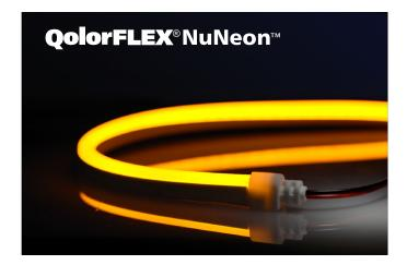
QolorFLEX NuNeon, Amber N914-A-10 is a sealed LED linear product that is flexible and safe for indoor or outdoor use. It is rugged, outdoor-rated, and dimmable. It can be cut to length and is available in a variety of colors plus RGB. It offers nearly the same visual impact as traditional blown glass neon without the problematic issue of installation and maintenance. QolorFLEX NuNeon operates on 24VDC and can be powered and controlled by a variety of QolorFLEX Dimmers and power supplies.
